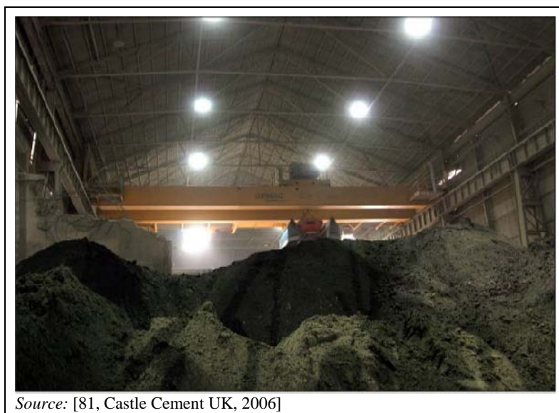
Figure 1.5: Example of covered raw material storage
