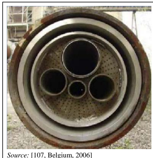
Figure 1.11: Example of a multi-channel burner
