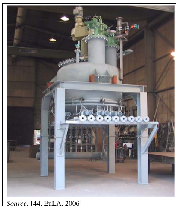
Figure 2.11: Example of a shaft kiln dosing system
